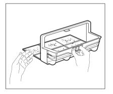
**5.** Lift the primary filter. Hold the heat exchanger filter and pull it out from the bottom compartment.
